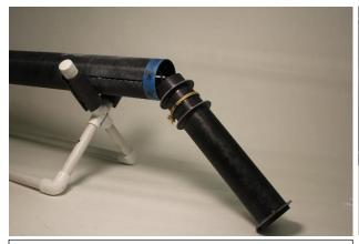
Step 7: Place tape around the booster, more time spent on preparation is less on clean up. Place epoxy around every centering ring.
