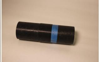
Step 13: The next thing to do would be to work on the av bay/electronics section. You will need to take the 2" switch band and the 9" coupler, tape one end of the coupler off, and make a line 3.5" in from both ends. Lightly sand the area between the lines, add a thin line of glue all the way around, sliding the switch band over it, always be prepared to remove any glue residue from this.
