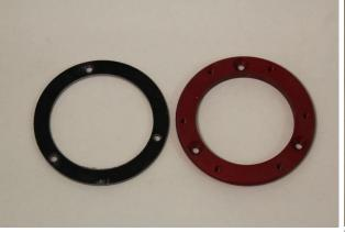
Step 3: Take one of the other centering rings, and the red aluminum thrust plate, stack them on top of each other evenly centered. Using a 1/8" drill bit, drill through the 3- countersunk holes into the centering ring, this will be the rear centering ring.
