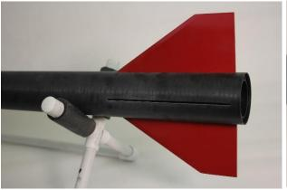
Step 9: Take the fins, one at a time, and glue them in with a bead of glue at the bottom, 10-minute epoxy is recommended here to hold them down and use rocket poxy for the fillets. When gluing the fins, make sure they are perfectly straight by using a guide or looking down the rocket to ensure it flies properly.
