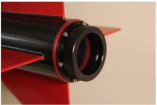
Step 15: Take the red aluminum thrust plate and the 3, 8-32 Screws and thread them into the rear centering ring, you may need to use a tap to get it to bite good. Adding a bit of glue on the threads will help if they strip or for a permanent fit. After this, take your Aeropack Flanged Retainer and screw it onto the thrust plate securely. Congratulations your rocket is now done! Feel free to contact us for any questions regarding decal installation or the rocket kit assembling.
