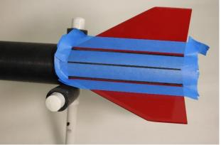
Step 10: Once all 4 fins are secure, tilt the rocket so both fins are off to the side equally. Place tape roughly 3/16" away to create a nice small fillet, also place tape at the front and back of the fillet to prevent a runoff.
