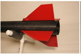
Step 11: Remove the tape from fillets 30-40 minutes after when the glue starts to set up. You will need to do this with all 4 fins, which will be 8 fillets total. When the glue is dry, take fine sandpaper and sand the fillets smooth.
