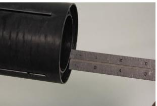
Step 8: Insert the motor mount assembly in, the rear of the tube needs to be exactly 1/8" in, to seat perfectly on the aluminum thrust plate. Clean the inside between body tube and motor mount with acetone, cleaning any glue residue sitting there. Let this dry before moving onto next step.
