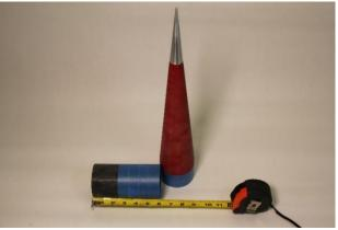
Step 12: Now the booster should be nearly complete. Take the 6" nosecone coupler and nosecone, tape 3.5" up the coupler, there should be 2.5" left, which will go into the nosecone. Sand this edge with rough sandpaper as well inside of the nosecone. Place a small amount of epoxy and slide the coupler into the nosecone.
