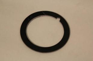
Step 2: Take fine sandpaper, around 200 grit and sand all 3 centering rings near the inner and outer edges, as well as the 4 fins on both sides about ¾" up from the root. Any part where glue is added, be sure the material has been ruffed up to ensure a tight bond with the glue. Then use a file and add a slight grove on one of the centering rings for the shock cord to pass through.
